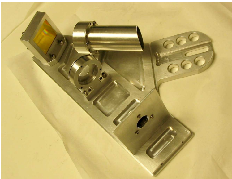
Figure 3. The baffles for the reimager at the top and the slit at the bottom of the image are to minimize stray light. This is especially important because the diffuser/lens in front of the slit floods the enclosure with light.
